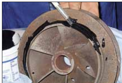
WEICON WR - Coating of a rotatory pump
