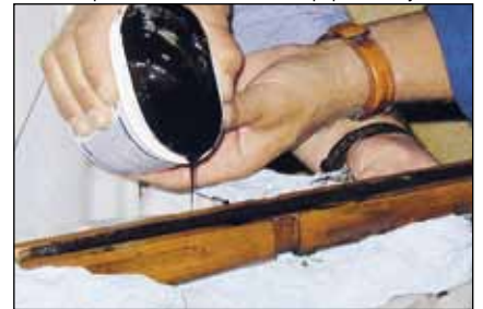
WEICON WR - Fixing of a rifle barrel to the rifle butt
